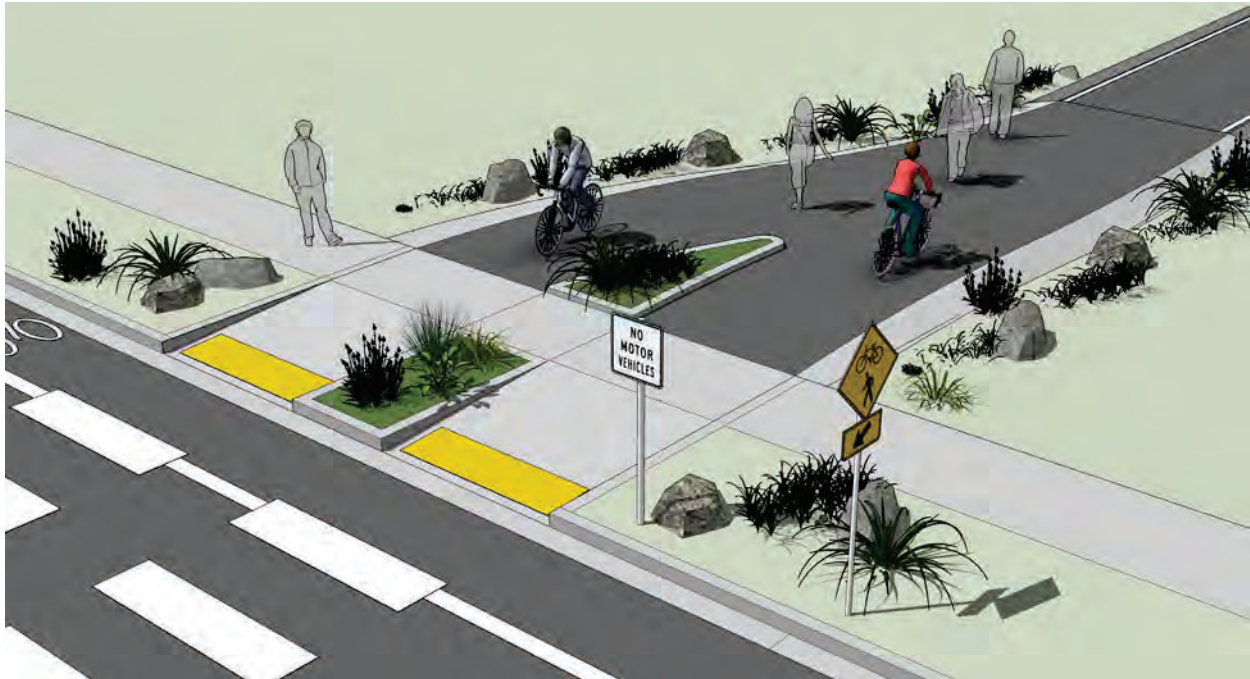
FIG. 4-22 ALTERNATIVE TO BOLLARDS AT ACCESS POINTS
