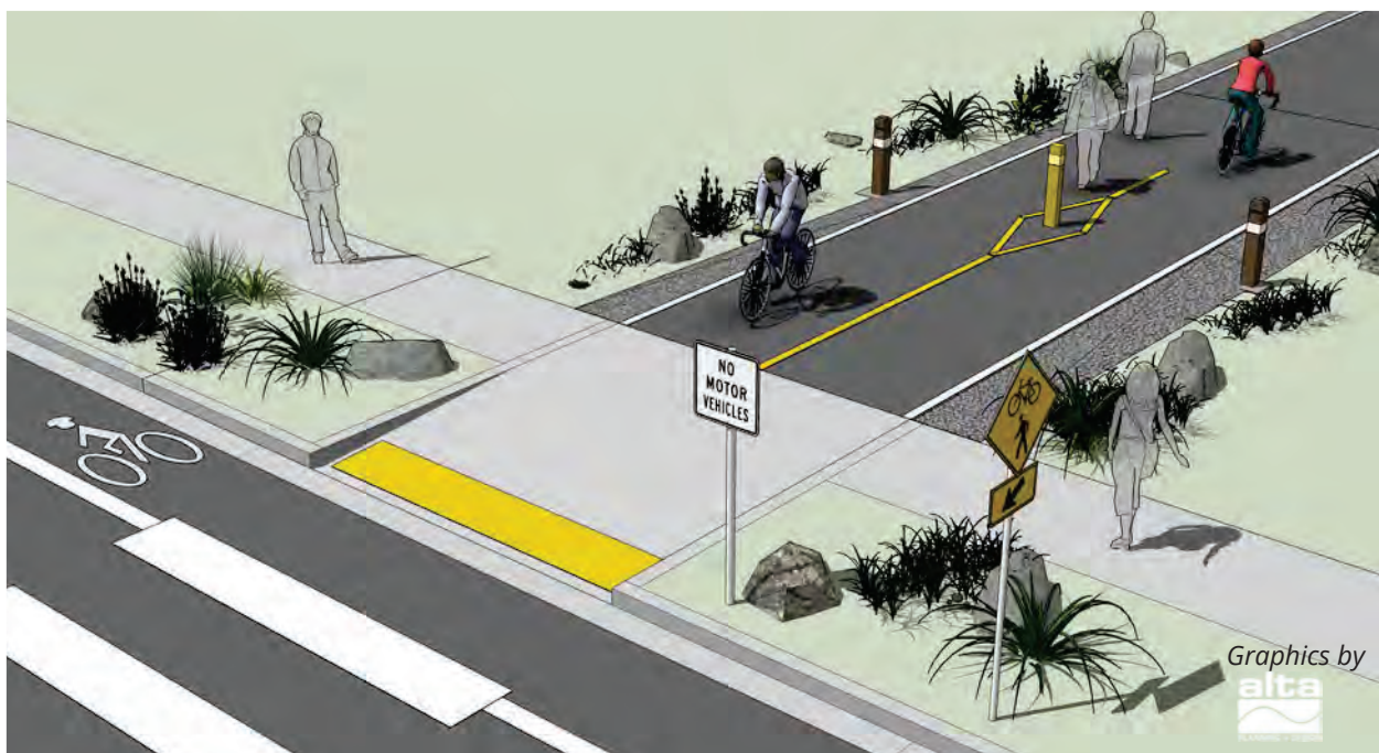
FIG. 4-23 BOLLARDS AT ACCESS POINTS
