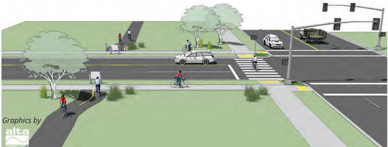
FIG. 4-11 FULL TRAFFIC SIGNAL
